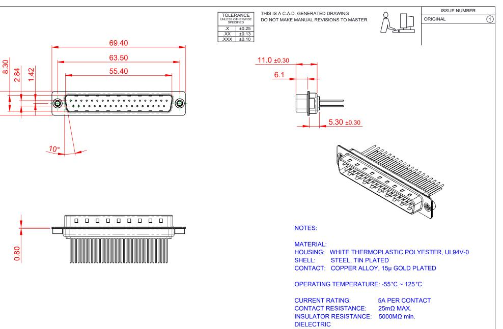
WITHSTANDING VOLTAGE: 1000V AC rms
