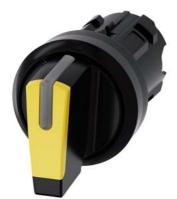
Selector switch, illuminable, 22 mm, round, plastic, yellow, selector switch, short, 3 switch positions I>O<II, momentary contact on the left, latching on the right, actuating angle 2x45°, 10:30h/12h/13:30h, with laser labeling, inscription or symbol Customer-specific selection with SIRIUS ACT configurator (CIN)
