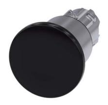
Mushroom pushbutton, 22 mm, round, metal, shiny, black, 40 mm, 3 switch positions, latches after pushing in, unlatches by pull-to-unlatch mechanism to center position, after pulling out the button Retraction to center position, with laser labeling, lower case
