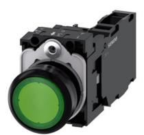
Illuminated pushbutton, 22 mm, round, plastic, green, pushbutton, flat, momentary contact type, with holder, 1 NO+1 NC, LED module with integrated LED 110 V AC, screw terminal, with laser labeling, upper case and lower case, always upper case at beginning of line
