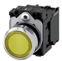
Illuminated pushbutton, 22 mm, round, Metal, shiny, yellow, pushbutton, flat, momentary contact type, with holder, 1NO, LED module with integrated LED 230 V AC, screw terminal, with laser labeling, lower case
