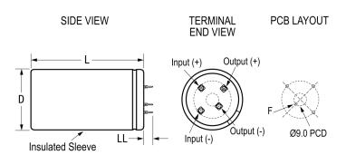
**General Information** Series ALN20S Dielectric Aluminum Electrolytic Description Audio Specific Aluminum Electrolytic Audio Grade Features RoHS Yes Lead 4 Pin Solder Tags AEC-Q200 No 125 g Component Weight Notes Dimensions D And L Include Sleeving.
