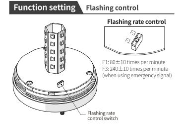
As a Flashing-only alarm light, it uses high luminance LED, which emits strobe light having excellent visibility in a long distance. Its visibility is superior in quality by using the specially developed dispersing lens, and it is suitable for tow truck and construction equipment.
