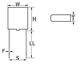
Dielectric MnO2 Tantalum Style Radial Molded Description Radial, Solid Tantalum, Molded RoHS Yes Termination Tin AEC-Q200 No Construction Molded Includes Standoff Height of 0.38 +/- 0.13mm. Miscellaneous Longest Lead Is Positive. Notes
