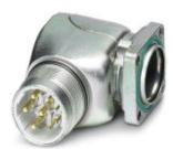
Device connector, front mounting, angled rotatable, for standard and SPEEDCON interlock, M23, number of positions: 4+3+PE, type of contact: Pin, Crimp connection, Axial O-ring, 4x Ø 3.2, shielded: yes, flange dimensions: 28 mm x 28 mm, Compatible with mating connectors with SPEEDCON or M23 standard knurled nuts
