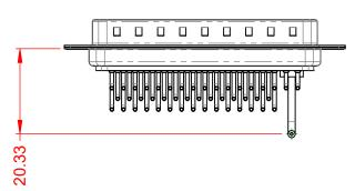
POWER/CO-AX CONTACT RATING:10A (CURRENT)(IF PRESENT)SIGNAL CONTACT CURRENT RATING:5A PER CONTACTSIGNAL CONTACT RESISTANCE:10mΩ MAX.INSULATOR RESISTANCE:5000MΩ min.DIELECTRIC5000MΩ min.
