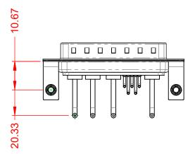
10A (CURRENT) POWER/CO-AX CONTACT RATING: (IF PRESENT) SIGNAL CONTACT CURRENT RATING: 5A PER CONTACT SIGNAL CONTACT RESISTANCE:  $10m\Omega$  MAX.
