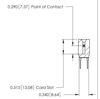
746 Series Ultra-Mate Card Edge Connector - Press Fit Part Number: 746-052-527-201
