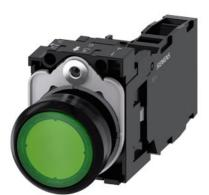
Illuminated pushbutton, 22 mm, round, plastic, green, pushbutton, flat, momentary contact type, with holder, 1 NO+1 NC, LED module with integrated LED 24 V AC/DC, screw terminal, with laser labeling, upper case and lower case, always upper case at beginning of line
