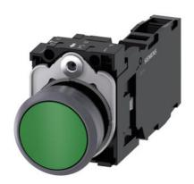
Pushbutton, 22 mm, round, plastic with metal front ring, green, pushbutton, flat, momentary contact type, with holder, 1 NO+1 NC, screw terminal, with laser labeling, inscription or symbol Customer-specific selection with SIRIUS ACT configurator (CIN)
