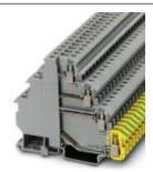
Sensor/actuator terminal block, connection method: Screw connection, cross section: 0.2 mm² - 4 mm², AWG: 24 - 12, width: 6.2 mm, color: gray, mounting type: NS 35/7,5, NS 35/15
