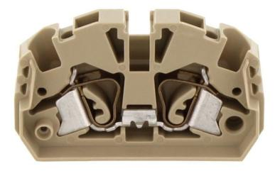
Feed-through terminal for direct mount, Tension-spring connection, Mounting type: Mounting surface, Rated cross-section: 2.5 mm<sup>2</sup>, Width: 11.1 mm, Colour: Beige
