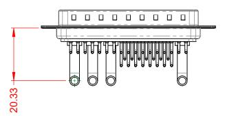
POWER/CO-AX CONTACT RATING: (IF PRESENT) SIGNAL CONTACT CURRENT RATING: 5A PER CONTACT SIGNAL CONTACT RESISTANCE:  $10m\Omega$  MAX. **INSULATOR RESISTANCE:** 5000MΩ min.
