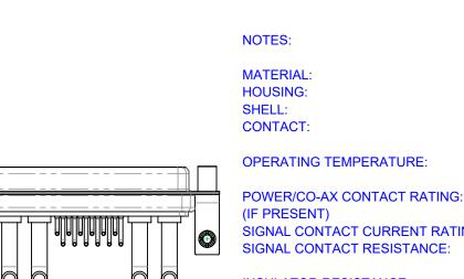
THERMOPLASTIC POLYESTER, UL94V-0 STEEL, TIN PLATED COPPER ALLOY, GOLD FLASH PLATED
