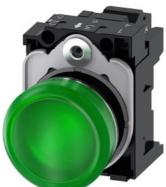
Indicator lights, 22 mm, round, Metal, shiny, green, lens, smooth, with holder, LED module with integrated LED 230 V AC, spring-type terminal, with laser labeling, lower case
