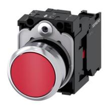
Pushbutton, 22 mm, round, metal, shiny, red, pushbutton, flat, momentary contact type, with holder, 1 NC, screw terminal, with laser labeling, upper case and lower case, always upper case at beginning of line
