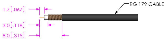
IN PROCESS 1 STRIP CABLE AND TIN INNER CONDUCTOR
