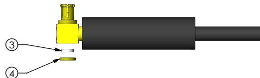
IN-PROCESS 6 PRESS INSULATOR AND CAP WITH CHAMFERED EDGE INWARDS
