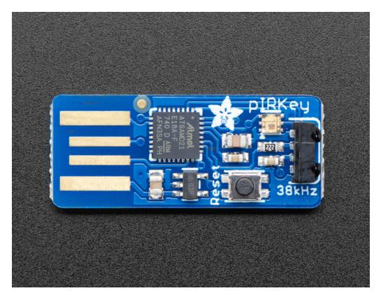
When you plug it in, the plRkey shows up as a triple device: USB disk drive to store code, USB serial for debugging and Python interactive command line, and USB keyboard/mouse that can transmit keypresses or mouse movements.
