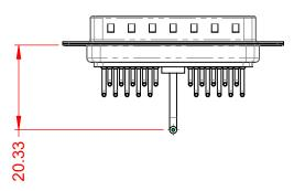
10A (CURRENT) POWER/CO-AX CONTACT RATING: (IF PRESENT) SIGNAL CONTACT CURRENT RATING: 5A PER CONTACT SIGNAL CONTACT RESISTANCE:  $10m\Omega$  MAX. INSULATOR RESISTANCE: 5000MΩ min.
