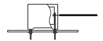
Temperature monitored inside the capacitor.
