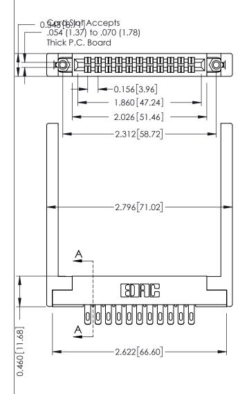
0.295[7.49] Card Slot SECTION 0.090[2.29] Point of Contact 305 ENG MASTER 305 / 315 / 355 Card Edge Connector
