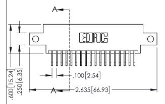
INSULATOR MATERIAL: THERMOPLASTIC PBT BLACK, UL 94V-0
