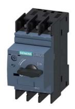
Circuit breaker size S00 for motor protection, CLASS 10 A-release 9...12 A N-release 163 A ring cable lug connection Standard switching capacity
