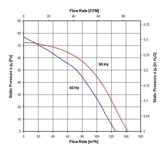
Measured with Traverse, 4000 TZ series. Nozzle is set at middle of the rotor.
