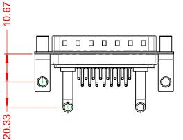
40A (CURRENT) POWER/CO-AX CONTACT RATING: (IF PRESENT) SIGNAL CONTACT CURRENT RATING: 5A PER CONTACT SIGNAL CONTACT RESISTANCE:  $10m\Omega$  MAX.
