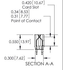
717 Series Ultra-Mate Card Edge Connector - Press Fit
