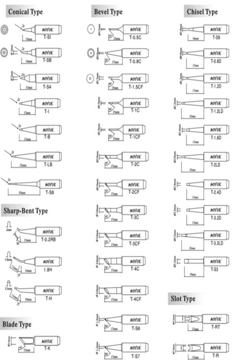
Suitable for all AOYUE soldering irons except lead free composite tip series, induction series and 938
