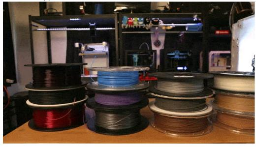
Although there is a wide range of filament types a 3D printer can handle, ABS and PLA plastics are by far the most popular. These two plastics are readily available in a staggering amount of colors, even glow-in-the-dark!
