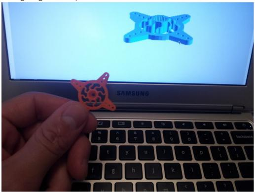
In order to produce 3D printer compatible objects, it is important to understand its limits. I like to think of a 3D printer as a spaghetti machine. It carefully stacks noodles on top of each other, and if there isn't enough noodle to stack on, it droops. The following three design elements can be implemented to help prevent drooping and will allow you to successfully print overhangs.
