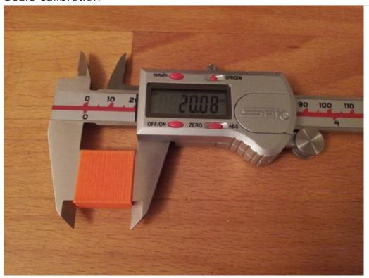
Scale calibration illustrates the process in which you compare the desired dimensions with the actual dimensions your printer produces. The easiest method for accomplishing this is to start by printing a calibration object, like a Calibration Cube (https://adafru.it/cos) or the Calibration Vector (https://adafru.it/cot). Once complete, use a set of calipers to check the dimensions and record your results.
