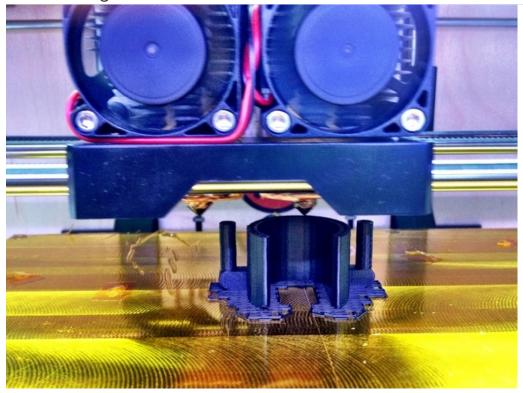
The build surface needs to be level to ensure the filament properly sticks to the surface and to provide a secure foundation for the print job. The bed can be leveled by either mechanically leveling the bed or using a raft to accommodate for unevenness.
