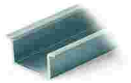
Item no.: 210-506 Steel carrier rail; 35 x 15 mm; 1.5 mm thick; 2 m long; unslotted; galvanized; similar to EN 60715; silver-colored
