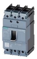
circuit breaker 3VA5 UL frame 125 breaking capacity class M 35kA @ 480 V 3-pole, line protection TM210, FTFM, In=70A overload protection Ir=70A fixed short-circuit protection Ii=10 x In UL489 SB (naval), 50 deg. cel. cable connection on both sides
