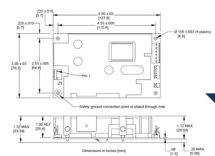
Note: Recommended standoff size is .375" high and all mounting hardware should be less than .28" in diameter. A standoff less than .375" high is acceptable when a thin insulator, 0.4mm thick (polyester, fish paper or equivalent UL rated 94V-2 minimum) is placed between the XR125 and the mounting chassis (refer to applicable UL standard for clearance requirements)
