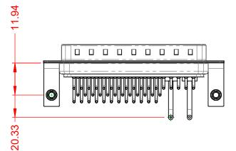
POWER/CO-AX CONTACT RATING: (IF PRESENT) SIGNAL CONTACT CURRENT RATING: 5A PER CONTACT SIGNAL CONTACT RESISTANCE:  $10m\Omega$  MAX. **INSULATOR RESISTANCE:** 5000MΩ min.
