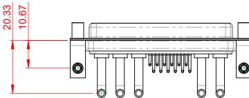
30A (CURRENT) SIGNAL CONTACT CURRENT RATING: 5A PER CONTACT
