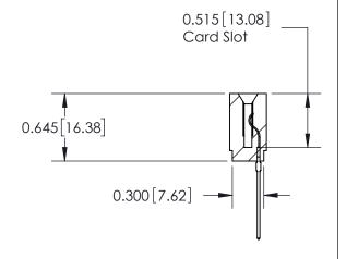
ACAD REFERENCE NO. 737 Series Ultra-Mate Card Edge Connector - Press Fit DRAWN: Part Number: 737-013-541-101 CHECKED: **EDAC INC** SCALE: THESE DRAWINGS AND SPECIFICATIONS ARE THE PROPERTY OF EDAC INC.,AND TORONTO, ONTARIO SHALL NOT BE REPRODUCED, OR COPIED DRAWING NUMBER CANADA OR USED AS THE BASIS FOR THE 737-ENG MASTER MANUFACTURE OR SALE OF APPARATUS YOUR CONNECTION TO QUALITY & SERVICE WITHOUT WRITTEN PERMISSION.
