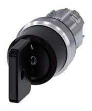
Key-operated switch O.M.R, 22 mm, round, metal, shiny, lock number 73034, black, with 2 keys, 3 switch positions I-O-II, latching, actuating angle 2x45°, 10:30h/12h/13:30h, Key removal I+O+II, Z=50-unit packaging
