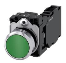
Pushbutton, 22 mm, round, metal, shiny, green, pushbutton, flat, momentary contact type, 1 NO+1 NC, screw terminal, with laser labeling, inscription or symbol Customer-specific selection with SIRIUS ACT configurator (CIN)
