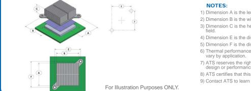
1) Dimension A is the length of the heat sink in the direction of the flow.
