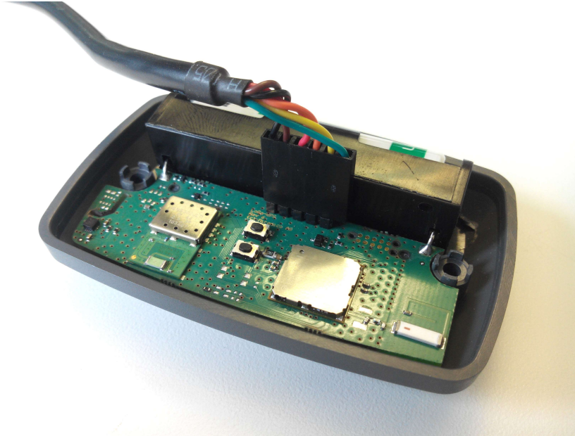
Illustration 4: FTDI Connect cable, connected to the tracker's pin header.
