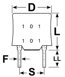
**General Information** Series SBCP-11HY Style Through-Hole Description Radial Leaded, Ferrite Power Inductors DC-DC Converters, Nickel-Zinc (NiZn) Ferrite Core Features RoHS Yes Lead Wire Leads Core Ferrite Contains 4 Reels of 400 pieces each. Do Not Expose Notes To Direct Sunlight.
