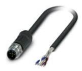
Bus system cable, CANopen<sup>®</sup>, DeviceNet<sup>™</sup>, 5-position, FRNC halogen-free, black, shielded, Plug straight M12, A-coded, on free cable end, cable length: 2 m, for outdoor applications, with high-grade steel knurl
