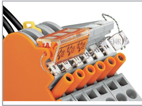
A lock-out seal can be used on the disconnect link in notched "I" position.
