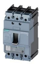
circuit breaker 3VA5 UL frame 125 breaking capacity class S 25kA @ 480 V 3-pole, line protection TM230, FTAM, In=20A overload protection Ir=20A fixed short-circuit protection Ii=7.5...15 x In UL489 SB (naval), 50 deg. cel. cable connection on both sides
