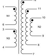
N2 denotes three windings connected in parallel. Terminals 7+8+9 and 10+11+12 must be tied as solder bridging is allowed.
