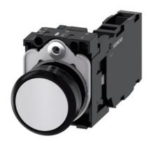
Pushbutton, 22 mm, round, plastic, white, pushbutton, flat, momentary contact type, with holder 1 NO+1 NC, screw terminal, with laser labeling, upper case and lower case, always upper case at beginning of line
