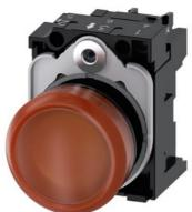
Indicator lights, 22 mm, round, plastic, amber, lens, smooth, with holder, LED module with integrated LED 110 V AC, screw terminal, with laser labeling, symbol number according to, ISO 7000 or IEC 60417
