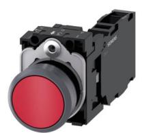
Pushbutton, 22 mm, round, plastic with metal front ring, red, pushbutton, flat, momentary contact type, with holder, 1 NO+1 NC, screw terminal, with laser labeling, upper case and lower case, always upper case at the beginning of the word
